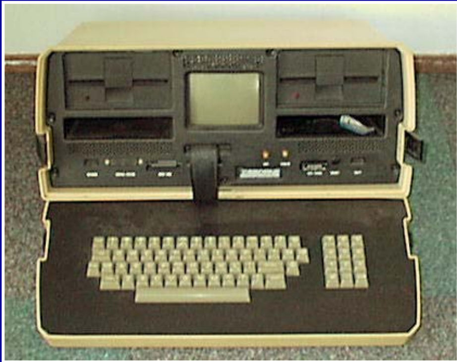
Osborne 1, ran CP/M, connections for printer & modem. Small 50 character screen. Circa 1984
