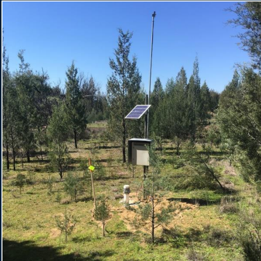
Tiltmeter measurement site, Bowen Basin, Australia
