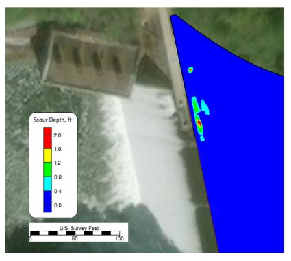
Measured Bathymetry  $\begin{aligned} \text{Max Scour} &\approx 2 \text{ feet} \approx 60 \text{ cm} \\ \text{Volume} &\approx 11 \text{ CY} \approx 8.5 \text{ m}^3 \\ \text{Cmax} &\approx 105 \text{ mg} \backslash l \end{aligned}$
