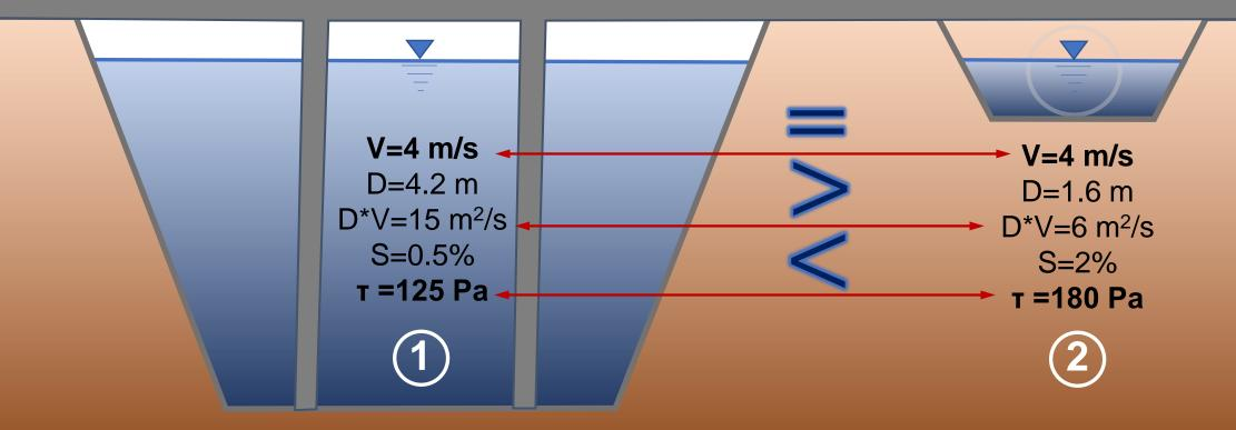
Velocity and shear stress for uniform flow
