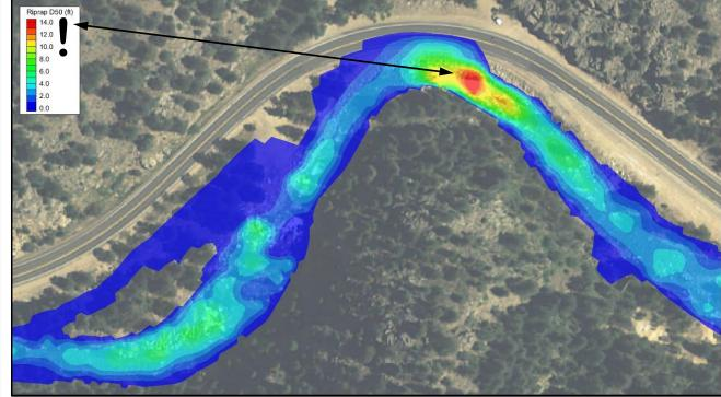
Figure 8.5. Riprap sizing contours based on 2D model depth and velocity results.
