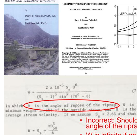
$\frac{0.27 \text{ U}^2}{(\text{S}_{e} - 1) \text{gD}_{\text{ED}}} = \sin (70^{\circ} - \theta)$
