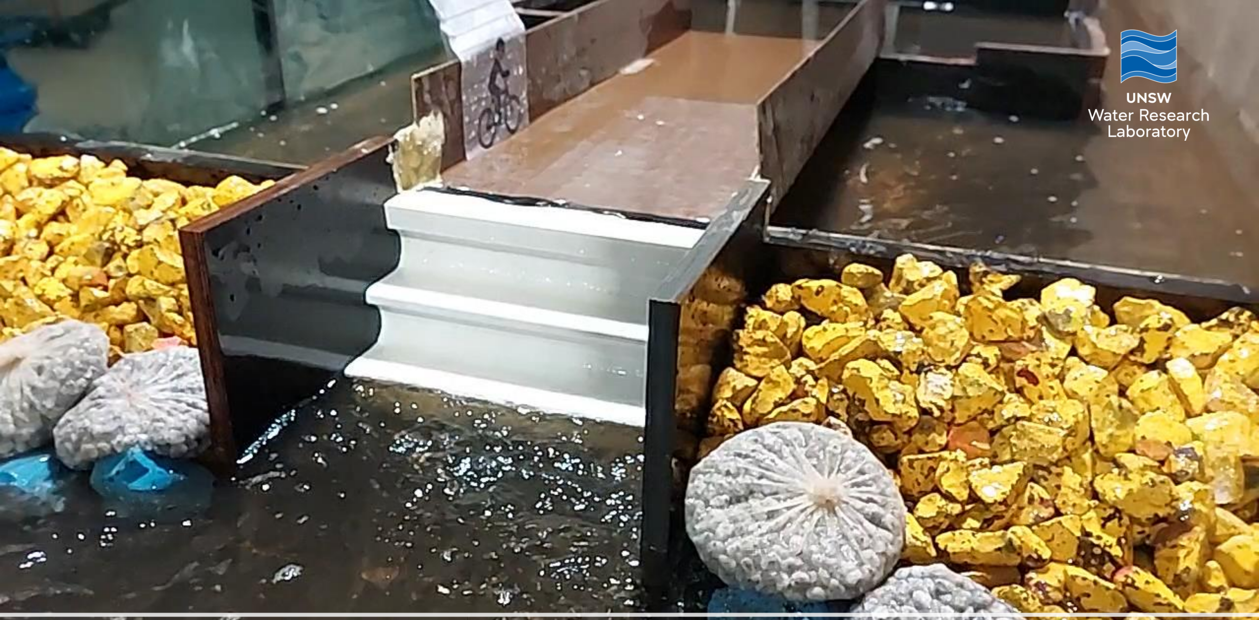
Stepped seawall design testing – 1.2 m wave flume
