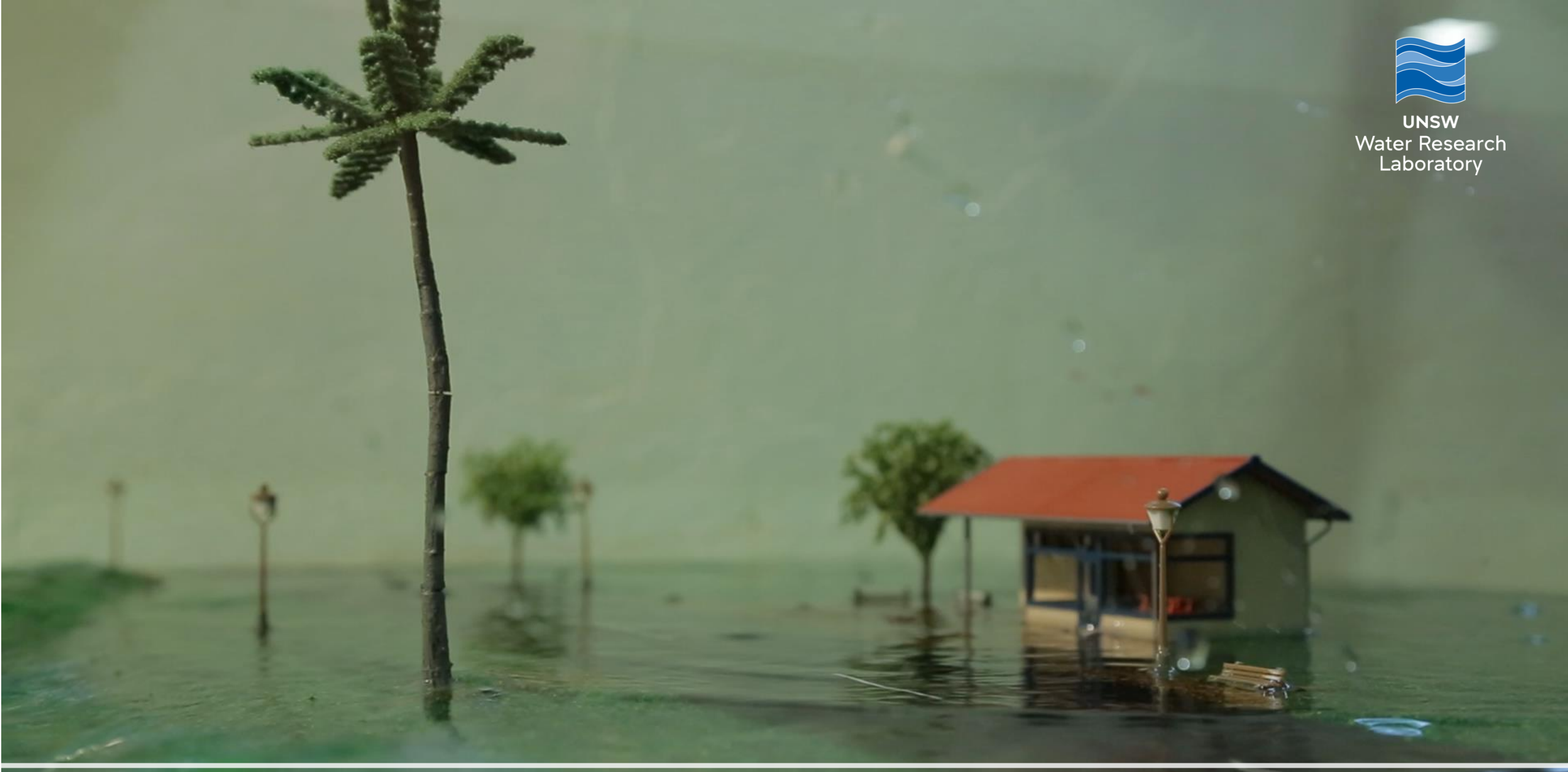
Physical modelling of a Pacific Island during a cyclone
